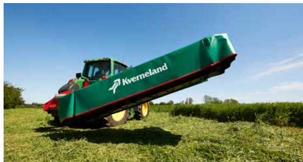
Lifting on headlands via hydraulic cylinder – ample ground clearance.
