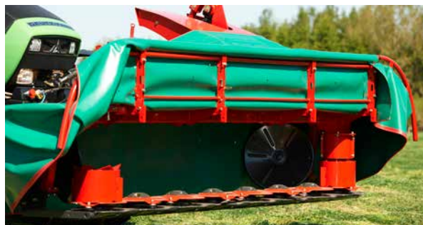
Easy access to the cutterbar with foldable front and side guards.
